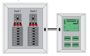
One possibile configuration is to mount the boards in an enclosure located under a raised floor. This can be a space-saving solution for facilities already crowded with equipment and wiring, such as data centers.
